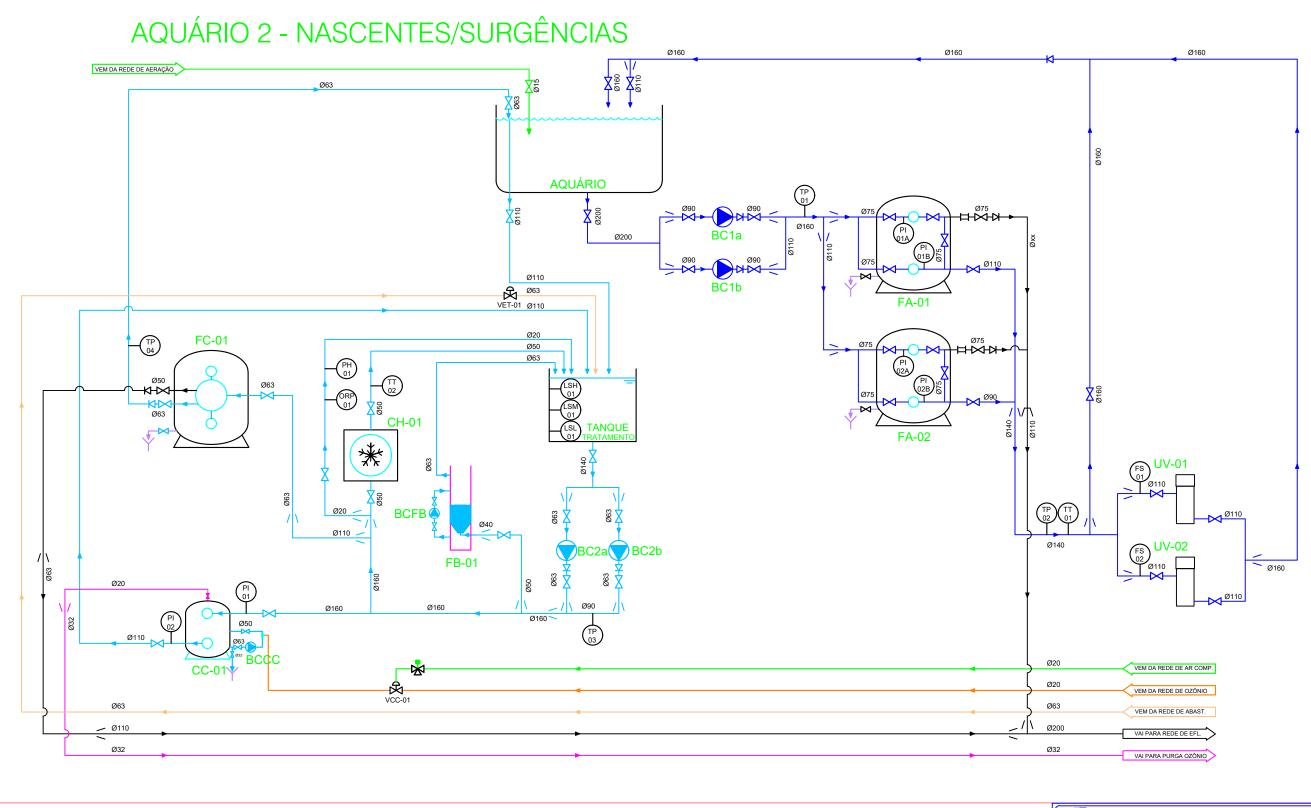
BOMBAS: BC1a - Bomba Maxin 4,5cv - 50Hz
