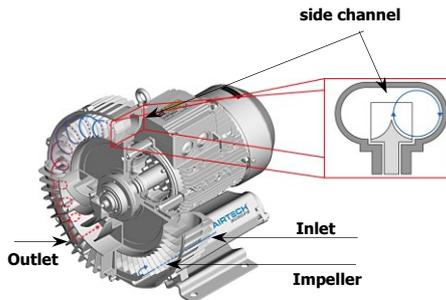
Two-stage machines have two side channels, each with one impeller connected in a series to achieve a better final pressure/differential pressure.
