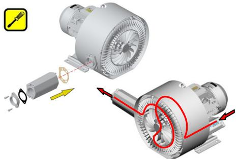
The discharge silencer for double stage side channel blowers acc. 3.) is supplied apart and has to be installed before startup. Do not remove factory mounted metal covers!
