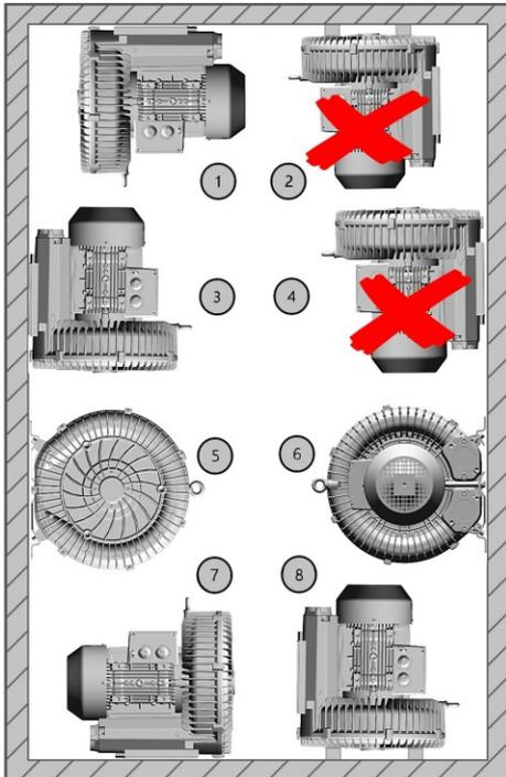
**2 4** Installation of the side channel blower in the vertical axle position with the motor facing downwards is not permitted on the wall or on the ceiling.
